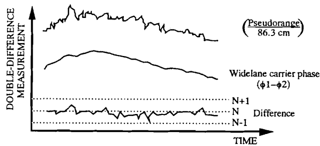
Fig. 5. Use of pseudorange for resolving the integer-cycle ambiguity in the widelane carrier phase data ( \phi_1 - \phi_2 ). The wavelength for widelane phase is 86.3 cm. This method is independent of baseline length [Melbourne, 1985].
