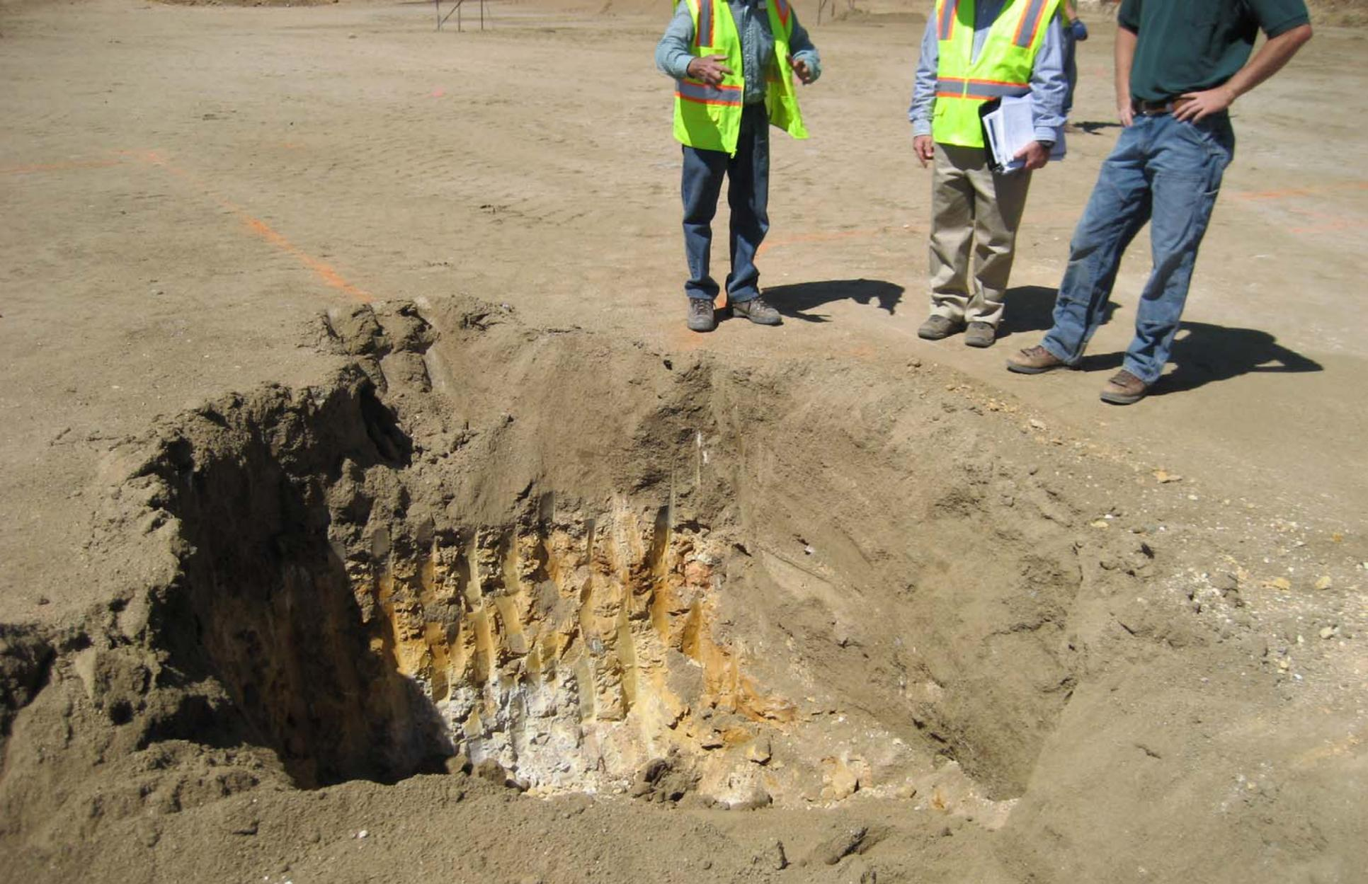
Hole for septic sump, 12 June 2008, illustrating 2 feet of decomposed granite above hydrothermally altered andesite
