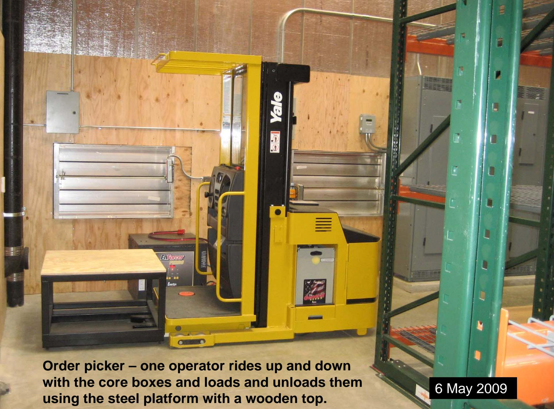
**Order picker – one operator rides up and down with the core boxes and loads and unloads them using the steel platform with a wooden top.**
