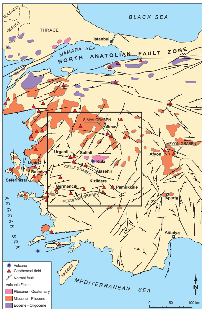
Figure 2. Generalized geologic map of western Turkey showing major fault zones and locations of geothermal systems. Black box surrounds the study area. Note the lack of Quaternary volcanism in the region. The mantle-derived basalts of the Kula volcanic field are the only Quaternary volcanics in the region.
