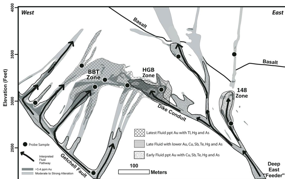
**Figure 1.** East-west cross-section 60300N looking north, illustrating relationships between, alteration, mineralization and structure. Note the close correlation between alteration and Au grades >3.4 ppm. Arrows indicate interpreted ore fluid pathways based on pyrite chemistry analyses (black circles mark analysed sample locations).
